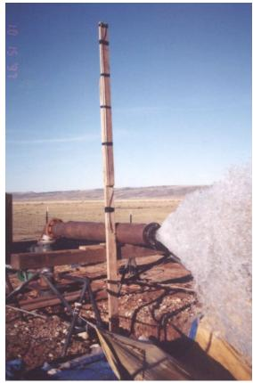
Spur No. 2 aquifer test: This well yielded 1,400 gpm for 30 days.
